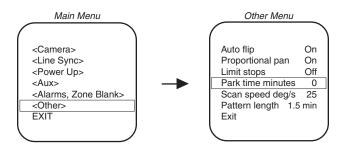
This feature causes the dome to park at preset 1 after a programmed number of minutes of control inactivity. The time can be set from 1 minute to 720 minutes (12 hours), or it can be set to zero, which disables this feature.
